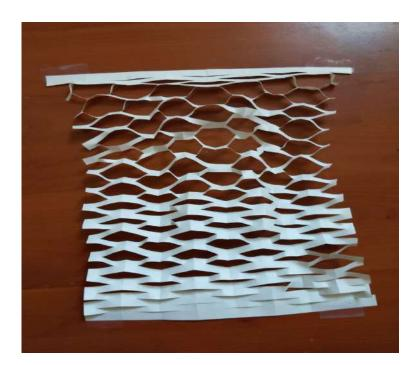
You can make quite the pattern with this technique! It's very useful as well to engineers. Some mesh and metal fencing is manufactured this way because you can easily take a thin sheet of metal and punch a bunch of holes in it like this, and make it much longer! What other applications can you think of for this pattern?
